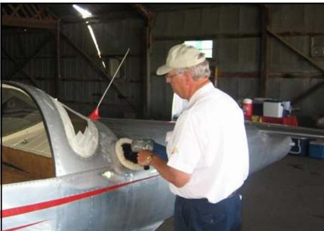
1. Using Nuvite NuShine II Grade F9, put big wet “fingerprints” of polish every 3” over a 2’ X 1 ½’ area to be compounded. Compound buff using a variable speed circular (“car”) buffer and 100 % wool “compounding” pad. (Nuvite EQ-140 or 3M #05711). “Compounding” pads can be identified by the tufted pad face that is “twilled” into tufts, similar to a cut-pile carpet. **VERY IMPORTANT:** Do not use standard “loose wool” pads.
