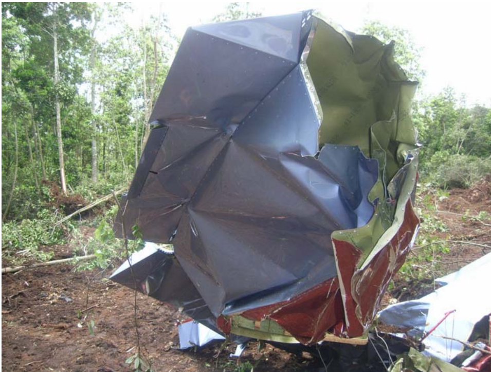
Right wing, lower surface, no apparent buckle at inboard end of aileron, other buckle may be due to leading edge impact.
