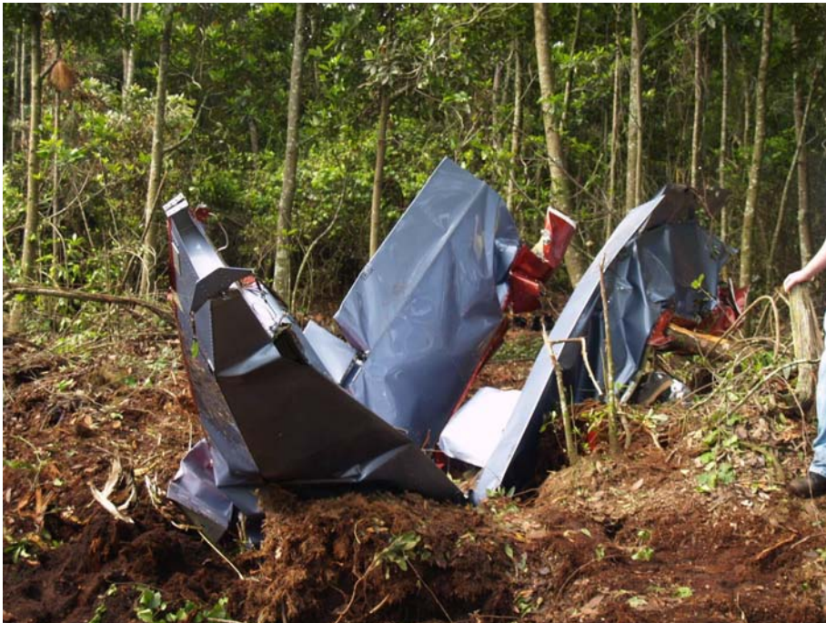
Left wing wrapped around fuselage
