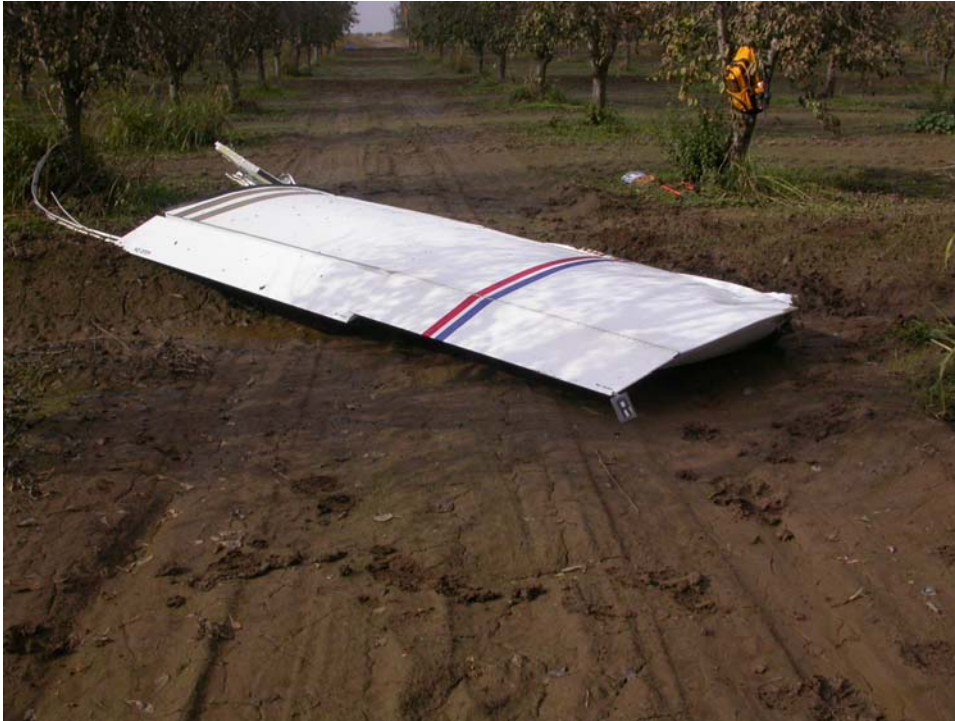
Right wing, top surface. No damage noted.
