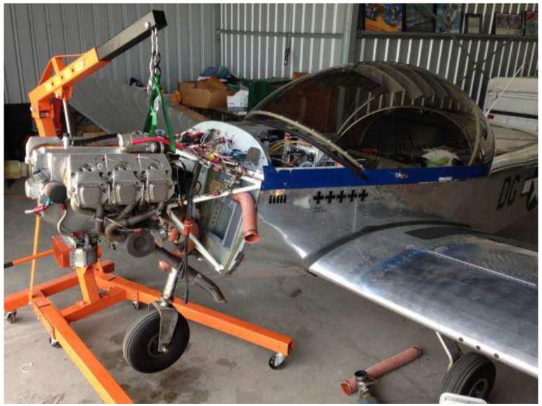
Used borrowed engine hoist to lift up on the engine mount
