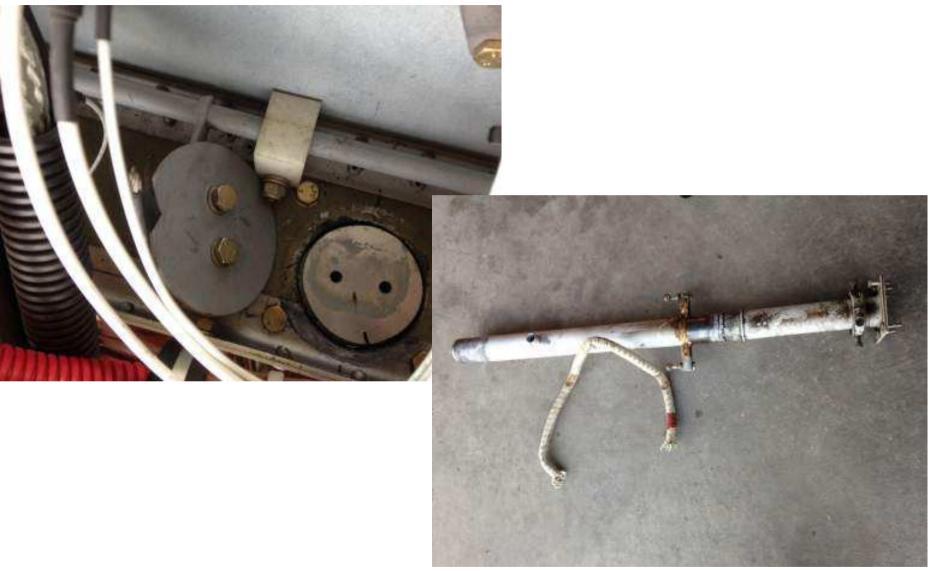
Removed gear leg cap, cut old bungee and pulled out entire gear leg.
