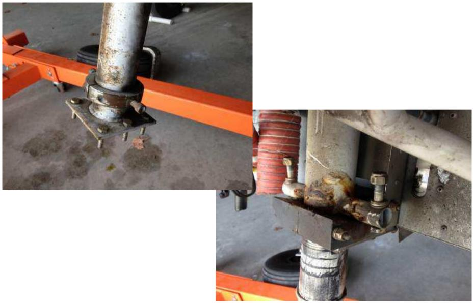
Removed nose wheel fork and disconnected steering and nylon bearing
