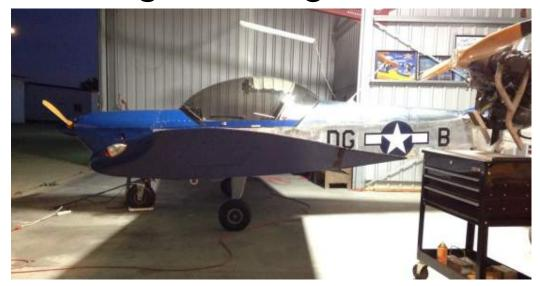
Slight nose down attitude noted, lose about 3.5" of strut length with broken bungee
