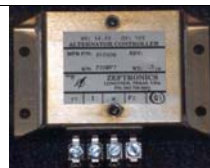
Figure 2 ACU that combines Voltage Regulation, OV Protection, Low & OV Sensor
